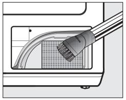
■ Vacuum up any soiling **carefully** using a vacuum cleaner dusting brush or small crevice nozzle.
